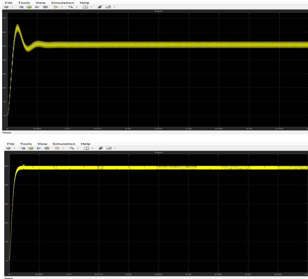
Figure 9. Open-loop and closed-loop Output voltages of Boost Converter
